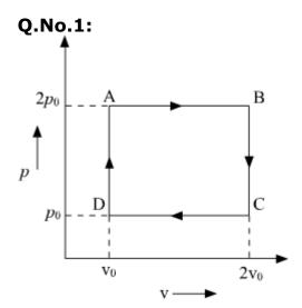
The above p-v diagram represents the thermodynamic cycle of an engine, operating with an ideal monoatomic gas. The amount of heat, extracted from the source in a single cycle is:
